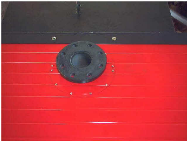
Raccordement au circuit hydraulique
