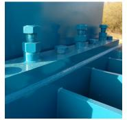
The **Galaxy** 2R narrow model features an adjustable shear beam that enables you to adjust the shear blades from the exterior of the machine. (Optional on 2R15ON and 2R19ON)
