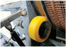
4WD for the drum screen, this concept doesn't only considerably reduce abrasion and maintenance effort, it also enables drum change in record time and without tools.
