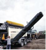
With this screen generation, the discharging belts have been revised consistently. This has not only enhanced the material flow, but it has also been put focus on the protection of the hydraulic
