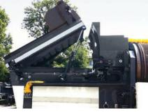
The additional disc screen system enables the separation of a third fraction and combines top-performance with maximum flexibility.
