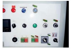
Full variability with as little buttons as possible. With our intuitive control panel the speed of the drum and the conveyors can be adapted perfectly to the various materials.
