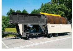
Open access to the motor, the hydraulic system and the drum considerably facilitates maintenance, cleaning and drum change.
