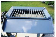
The TTS 520 can additionally be equipped with a stone grate or a vibro grate to remove large debris out of the sieving.
