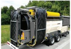
The TTS 520 is an all-purpose drum screen with an innovative Load Sensing System for minimum fuel consumption.
