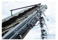
The side conveyor as well as the rear conveyor are offered in two different lengths and are available in 3,500 mm and 5,000 mm.
