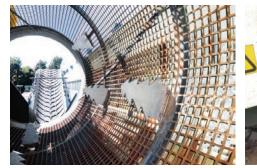
No auger in the drum, no forced conveying – in order to guarantee an optimum output quality with varied materials, the drum tilt, as well as all of the drivetrains are individually adjustable.
