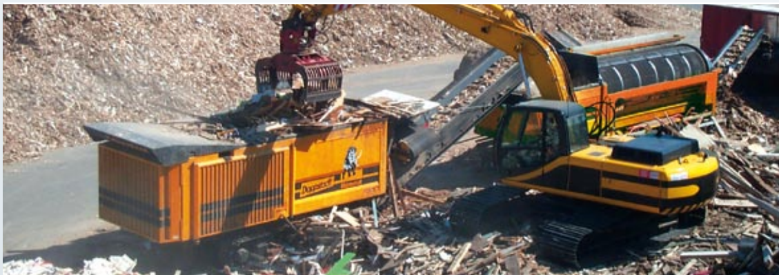
Waste wood processing with DW 3080 K and SM 720
