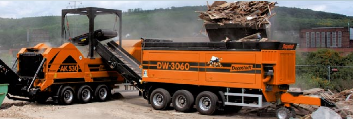
Shredding of waste wood/pallets
