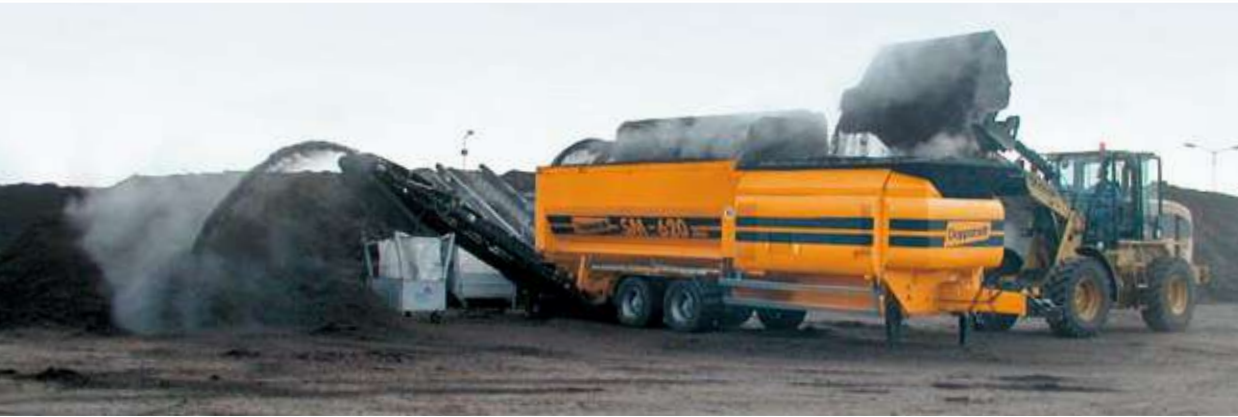
Composting: Separation via rear and side conveyor
