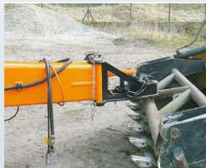
Displacing the machine by wheel loader
