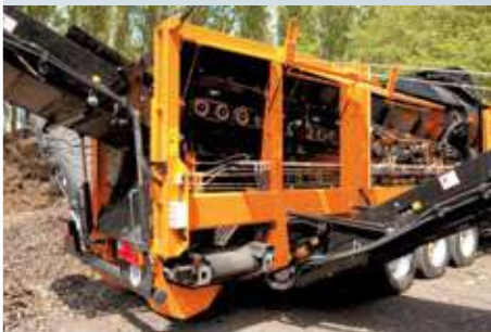
Two screening decks
